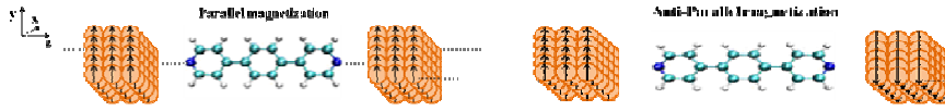
Fig. 1. A schematic representation of the FM/organic molecule/FM molecular junction in two configurations Parallel (P) and Anti-Parallel (AP) magnetization.
