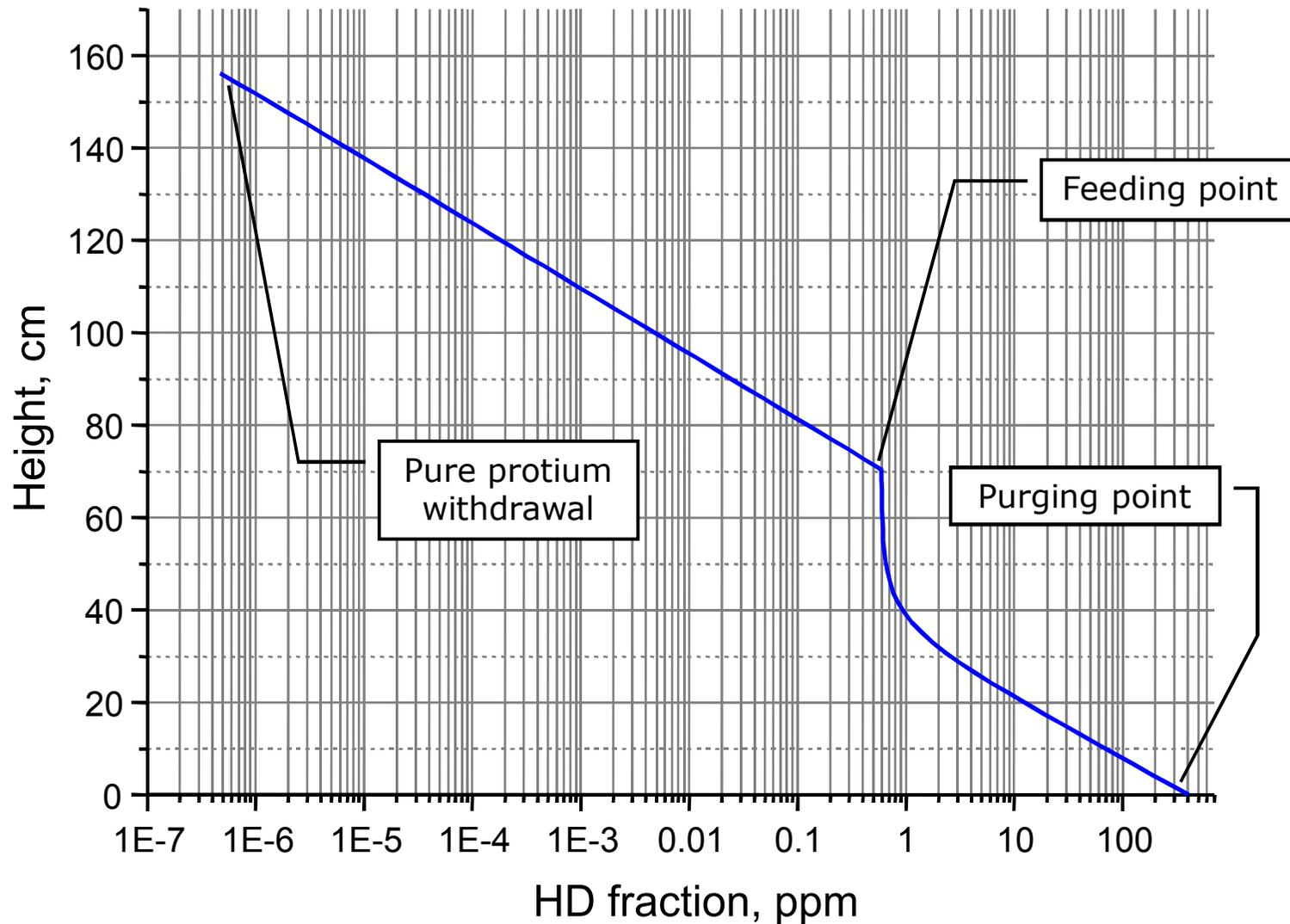
Feed flow rate = 1 L/min; Pressure = 1.5 bar; Purging flow rate = 0.015 L/min; HETP = 2.2 cm
