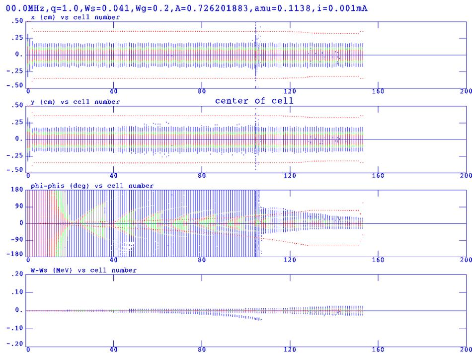
Beam envelopes for the RFQ design in the x, y, phase, and energy dimensions. Respective ordinate units are cm, cm, degrees and MeV. The colors blue to red show gradations in the intensity distribution.
