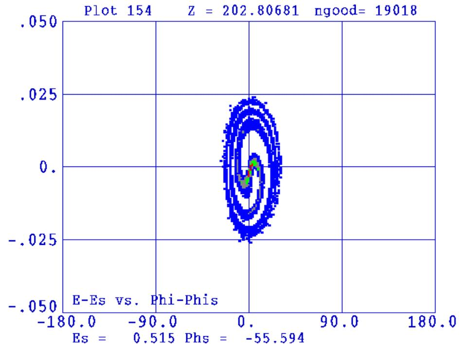
The phase-energy distribution for the RFQ output. Dimensions are in degrees and MeV.
