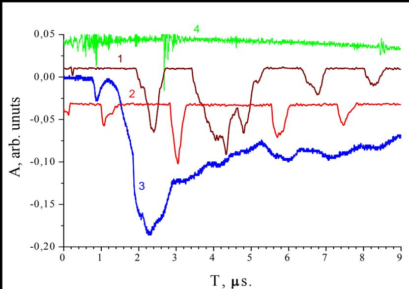
Waveforms of the: electron (1) and ion (2) currents from the spectrometer collector; (3) potential difference between electrodes #1 at figure of setup; (4) signal from neutron detector
