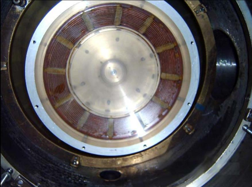
● Induction plasma source installed in the vacuum chamber of the accelerator
