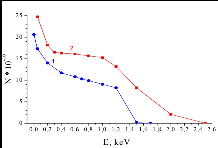
Integral spectra of ions (1) and electrons (2)
