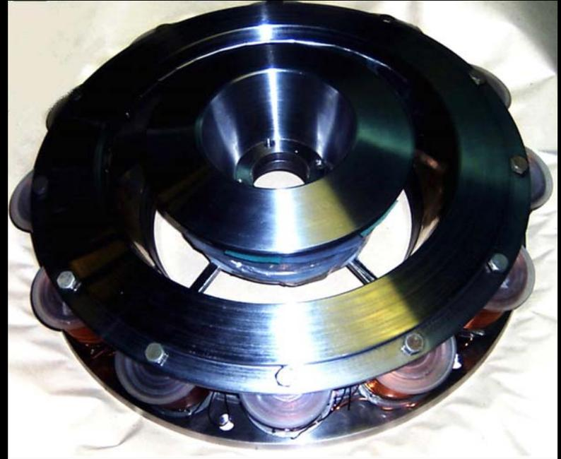
Electromagnet of the Hall ion source. The electromagnet is intended for generating a transverse isolating magnetic field in the accelerating gap.
