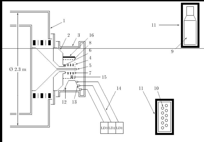
1 – high-current pulse generator; 2 – load unit of accelerator; 3 – diagnostic chamber; 4 – grid cathode; 5 – inverse current conductor; 6 – supersonic Laval nozzle; 7 – liner; 8 – current-intercepting rods; 9 – scintillation detector; 10 – thermal neutron detector; 11 – Pb shielding; 12 – light-cover cone; 13 – collimators; 14 – optical fibers; 15 – magnetic dB/dt probes; 16 – solid  $\text{CD}_2$  target; LD1, LD2 and LD3 – optical radiation detectors
