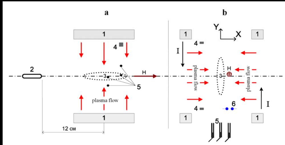
Schematic of experimental setup: a – view along B-field; b – side view normal to B-field
