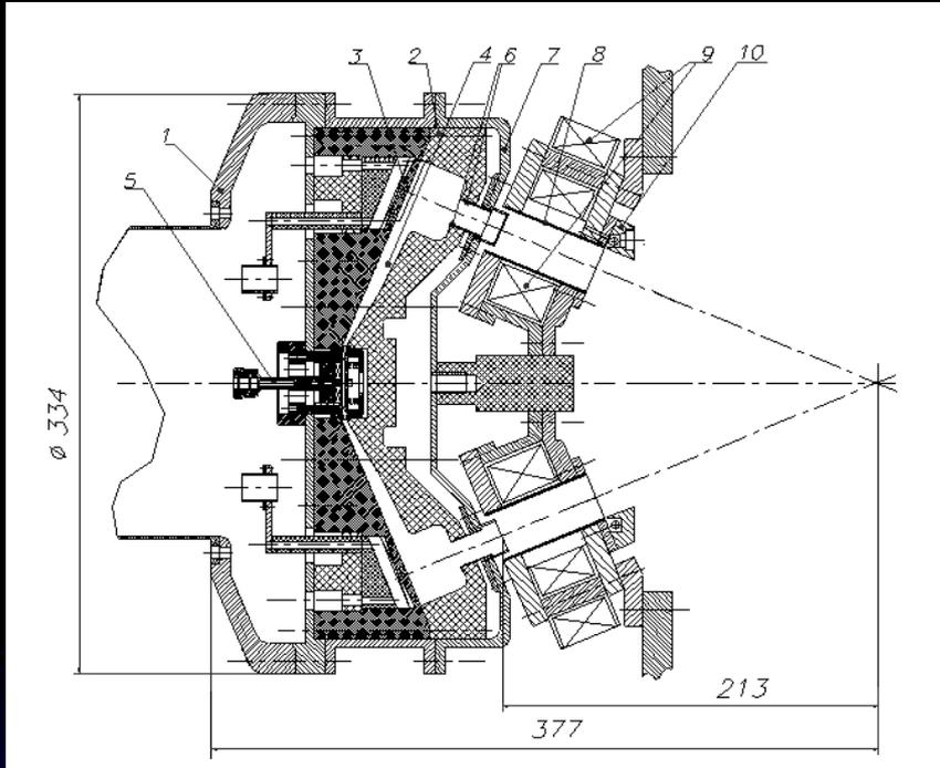
1 – anode holder, 2 – insulator, 3 – shock coil,
