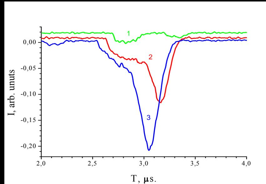
Waveforms of the collector current at different bias voltage of the grid
