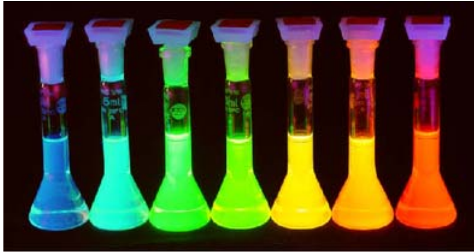
Fluorescence induced by uv-light in vials containing CdSe QD of different size
