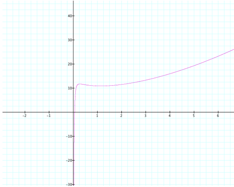
Fig.4. A temperature profile for cylindrical Couette flow, plotted against the horizontal radius, based on Eq.(6.1). The position of the walls is not indicated.
