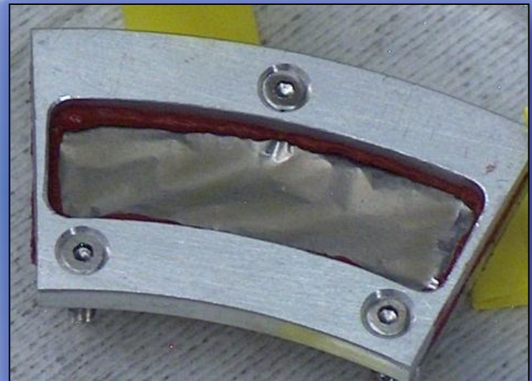
12 target sectors are in Dubna Average thickness 0.35 \text{ mg/cm}^2
