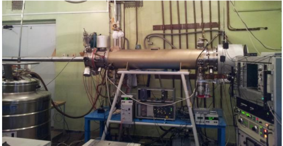
KRION-6T/ESIS has been assembled and being tested (March 2014)
