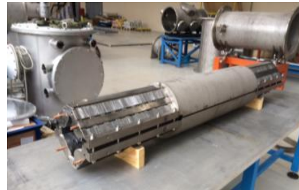
Sextupole corrector prototype for SIS100 and NICA Booster and its assembly
