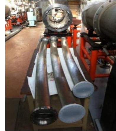
UH vacuum beam chamber (curved)
