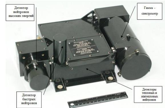
Mercurial Gamma-ray and Neutron Spectrometer (MGNS scientific instrument) is being developed to be placed onboard *BepiColombo* ESA interplanetary mission. MGNS project is multifunctional scientific instrument, comprising gamma-ray spectrometer and neutron detectors.
