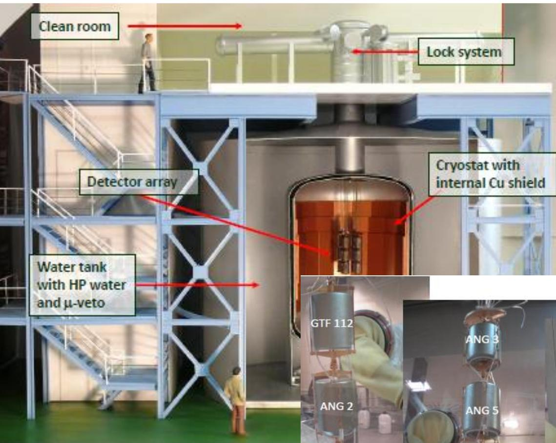
The array of high purity Ge detectors (8 enriched and 1 non-enriched) is installed inside the tank of LAr
